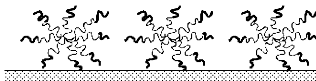
Figure 12. Scheme of copolymer micelles adsorbed on silica from C_6D_{12} solution.
